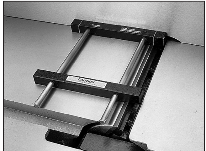
Figure 36. G1753 Jointer Pal® Knife Gauge.
